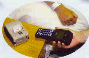
Scan patient wristband & transfer patient data to SATO MB200i and print sample label
