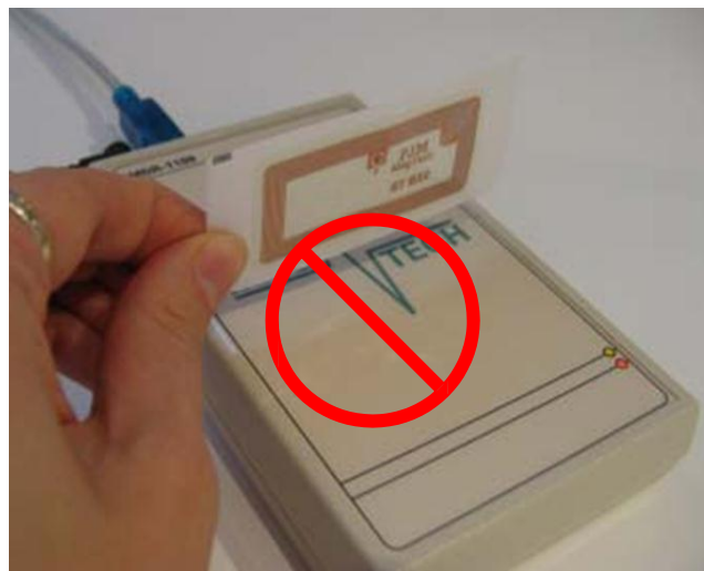
Incorrect orientation (90° angle).
