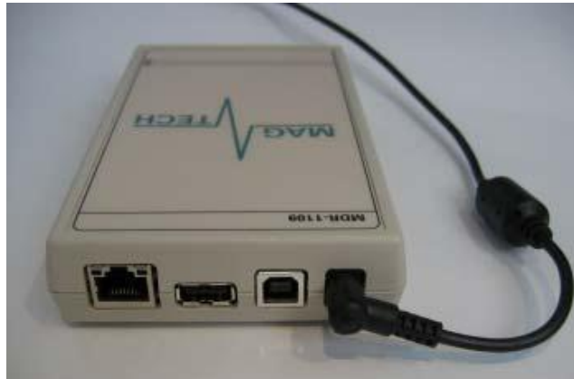
MDR-1109 with plugged-in low voltage power cable
