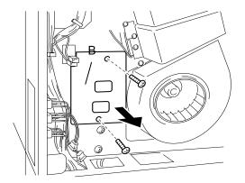
5. Remove the exit guide B by removing the two screws. (Figure E-4)
