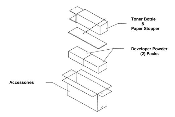
**Note:** Developer pack contains two (2) packages of developer powder each. Two packages of developer powder are used during initial printer prep.
