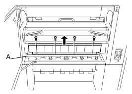
4. Remove the exit guide A by removing the four screws. (Figure E-3)
