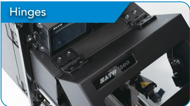
Larger hinges (when compared with legacy model) to provide extra strength for securing cover.
