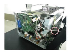
Remove two screws 6 and then remove the RTC bracket 7.
