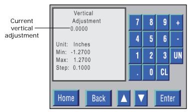
Figure 6-63. Vertical Adjustment screen.
