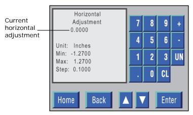
Figure 3-13. Modify Horizontal Fine Adjustment.
