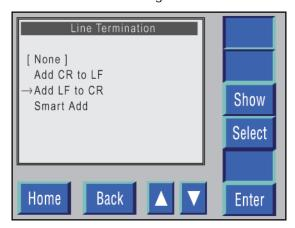
Figure 6-75. Line Termination screen.
