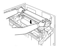
8. Re-install the OPC cartridge to its original position.
