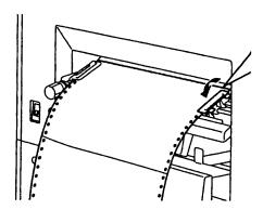
5. Adjust the width between the tractors to accommodate the form by rotating the knob D.
