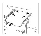
4. If the jam occurred at the exiting end of the tractor unit, separate the last usable printed page at the perforation, allowing it to drop onto the stacker table.
