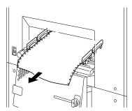
6. Close all open tractor covers. Raise the tractor unit by lifting up on the tractor unit handle.
