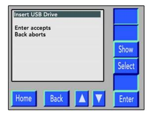
Figure B-38. Accept/Abort Install Configuration File option selected.
