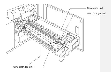
Figure 2-5. Components accessed from the EP holder.
