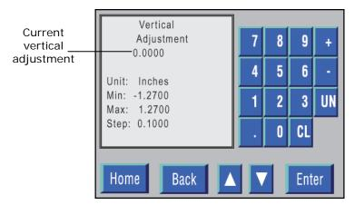
Figure 6-62. Vertical Print Adjustment screen.
