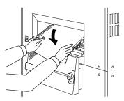
9. Open the lower tractor cover (and upper covers if used) and remove the documents from the belt.
