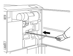
**Note:** If the transfer/charger lever is not completely inserted, the print image may be light.
