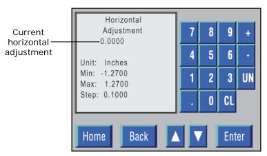
Figure 6-67. Horizontal Adjustment screen.
