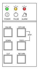
Figure 2-2. Top panel switches.
