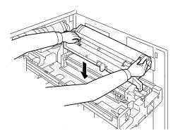
Note: To avoid damage, do not touch the OPC drum.
