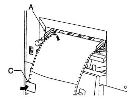
4. Load the stock on the right-side tractor (B) and close the cover.
