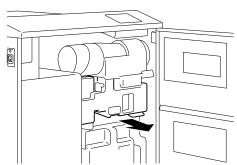
3. Remove the main charger unit by lifting up the developing unit side approximately 30 degrees (marked A).
