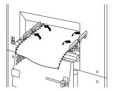
10. Separate the unloaded form, ejected form, and the form left inside the printer by cutting it along the perforation immediately before the tractor unit and after the exit area.
