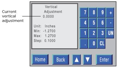
Figure 3-14. Modify Vertical Fine Adjustment.
