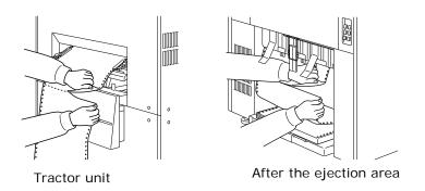
**Note:** When removing the jammed form, always pull it out in the feeding direction. Unfixed toner on the form can contaminate the interior of the printer.
