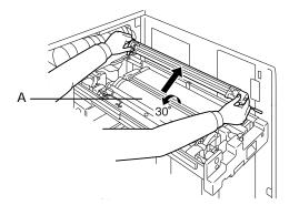
4. Remove the OPC cartridge by holding the handle and the plastic part (position B).
