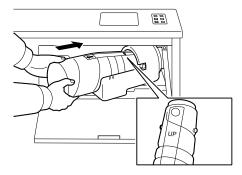
6. While holding the toner bottle in place, pull out the seal on the top face of the toner bottle.
