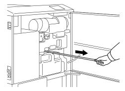
**Note:** When pulling out or inserting the transfer/separator lever, use caution to avoid bending it.
