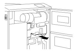
3. Remove the main charger unit by rotating and swinging up the developer unit side approximately 30 degrees (position A).
