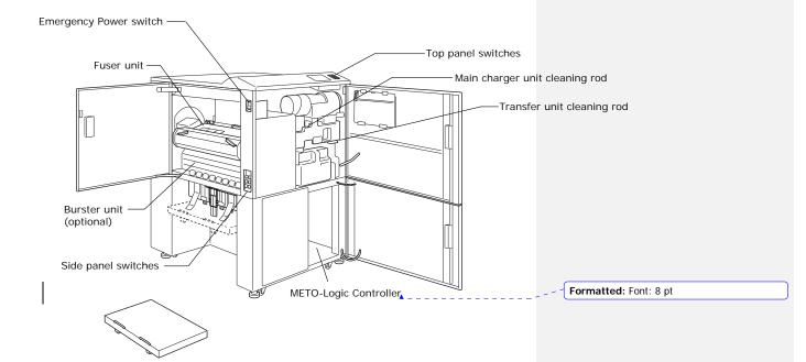
Figure 2-1. Left-side front view of LP 100R laser printer.
