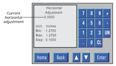
Figure 6-66. Horizontal Adjustment screen.
