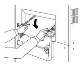
3. Open the lower tractor covers (and upper covers if used), remove the documents from the belt and, if the jam has occurred in this area, pull the jammed document out of the printer.
