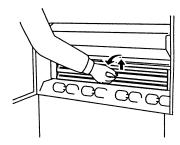
14. Remove the toner fuser filter and open the transport roller.
