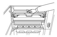
Use a cloth moistened with water to wipe off stains. If toner deposition has built up, use a neutral detergent.
