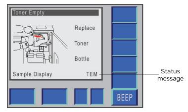
Figure 4-2. Control panel display for a status message.
