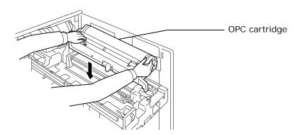
**Note:** To avoid damaging the OPC drum, make sure to re-install components in this order:
