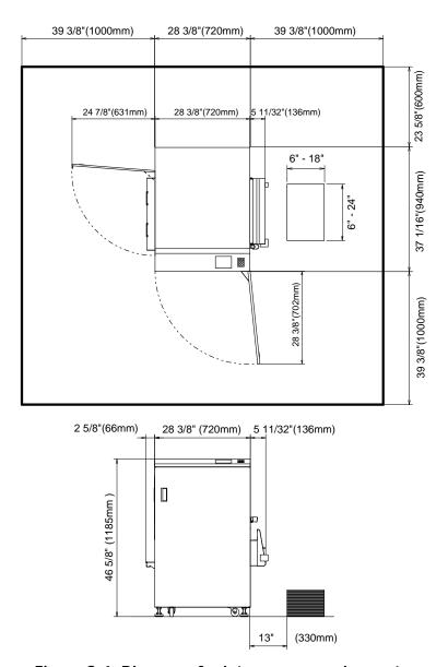
Figure G-1. Diagram of printer space requirements.
