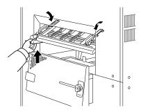
**Note**: Raising the tractor unit before closing the tractor covers will damage the covers.
