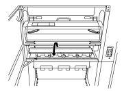
13. If the burster unit is enabled, open the burster area.
