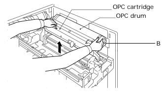
**Note:** Place the OPC cartridge on a level place, using a cleaning pad to protect the level surface and the OPC drum.
