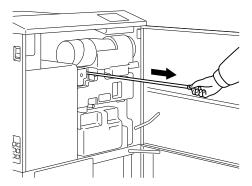
**Note:** When pulling out or inserting the charger cleaning lever, use caution to avoid bending it.
