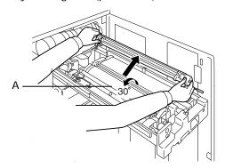
4. Remove the OPC cartridge by holding the handle and the plastic part (position B).
