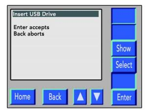
Figure B-53. Accept/Abort System Error Log Copy option selected.
