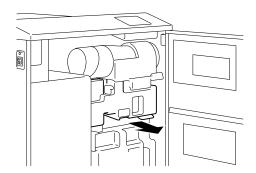
3. Remove the main charger unit by lifting up the developing unit side approximately 30 degrees (position A).
