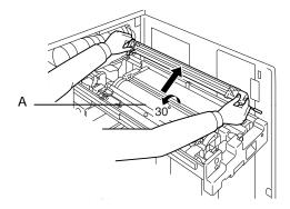
4. Remove the OPC cartridge by holding the handle and the plastic part (marked B).
