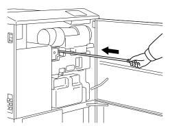
**Note:** If the charger cleaning lever is not completely inserted, the print image may display black streaks.
