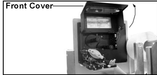
2. Pull the purple Head Lock lever upwards in a counterclockwise direction. The print head assembly will be lifted up to allow ribbon loading.
