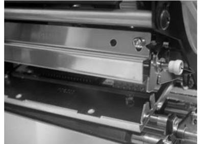
4. Pull the print head outwards and disconnect the two connectors attached to it.
