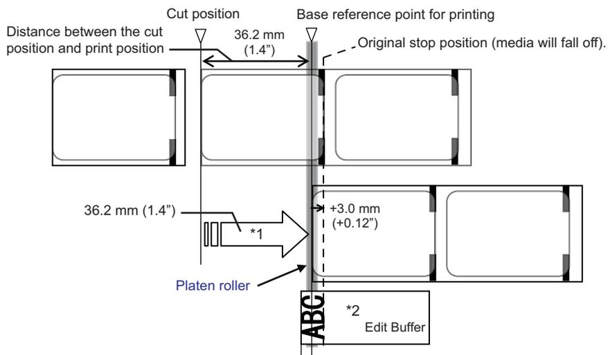
\*1. The original backfeed distance before adjustment is 39.2 mm (1.5"), however it is adjusted to 36.2 mm (1.4") in this case to prevent the media from falling off the platen roller area.
