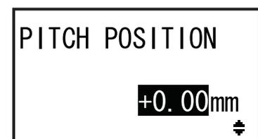
**3** Change the setting value. Press the  $\triangle/\nabla$  buttons to set the desired value.
