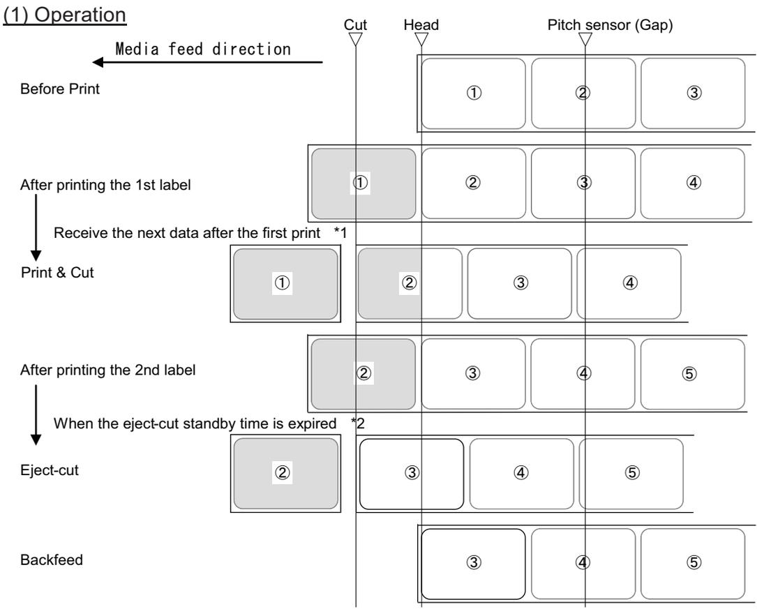
\*1 When the next print data is received after the first label is printed, the product prints the next data and cut the first one when it reaches the cut position.
