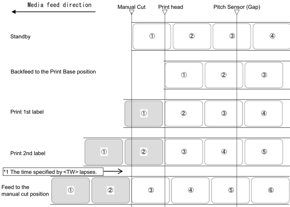
\*1 The media is fed to the manual cut position when time (option unit stand-by time; default value - 1000ms) specified by <TW> lapses and no print job is sent.
