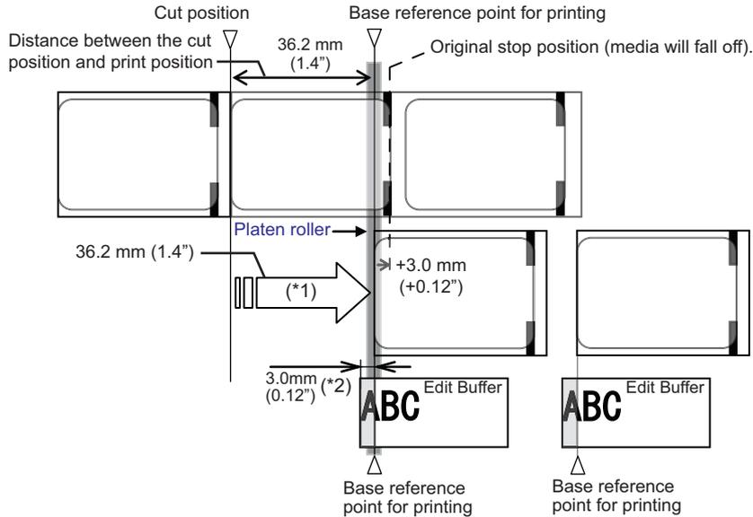
\*1. The original backfeed distance before adjustment is 39.2 mm (1.5"), however it is adjusted to 36.2 mm (1.4") in this case to prevent the media from falling off the platen roller area.
