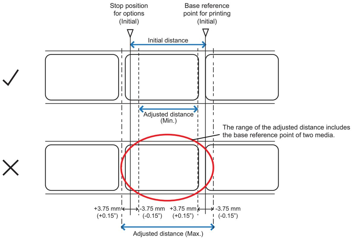
Adjustment range of the distance between the print position and the stop position for options:
