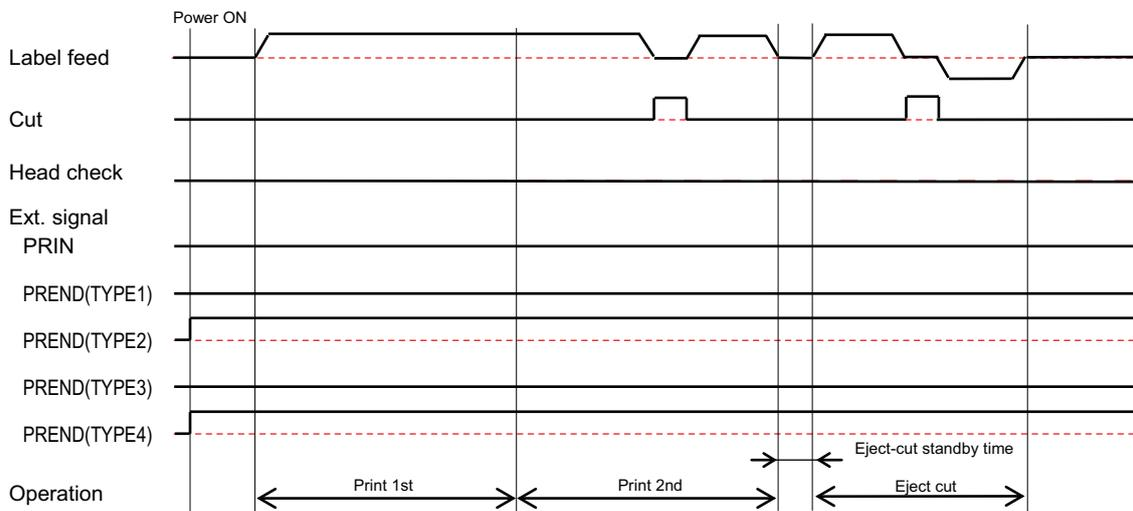
**8.7.13 No Pulse Input in Motion 3 Cutter Mode (Head Check Enabled)**
