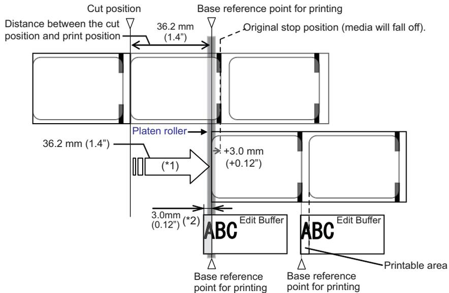
\*1. The original backfeed distance before adjustment is 39.2 mm (1.5"), however it is adjusted to 36.2 mm (1.4") in this case to prevent the media from falling off the platen roller area.
