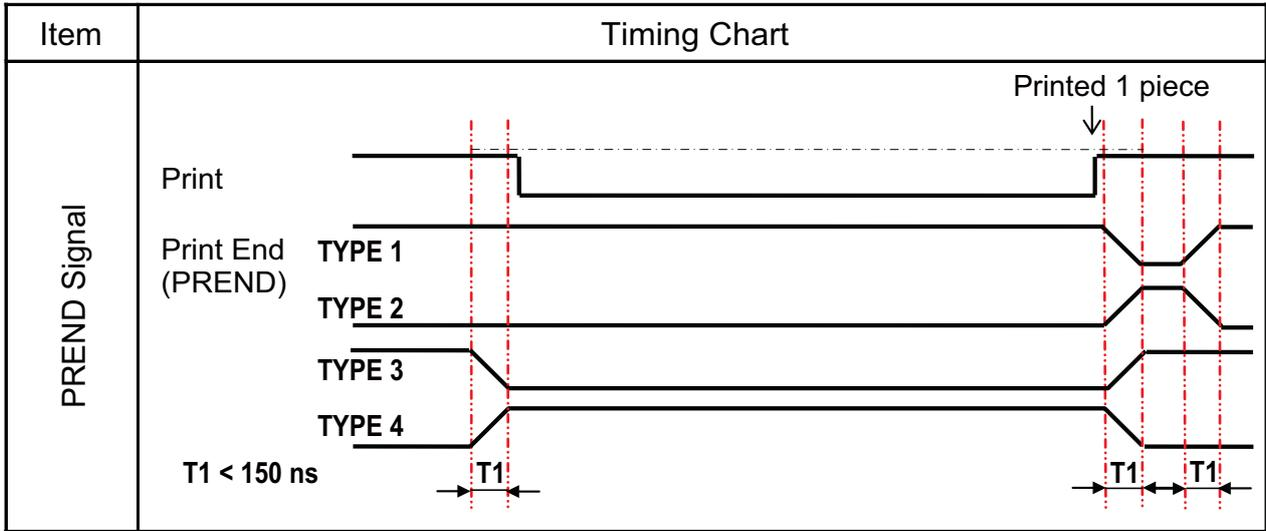
Rise or fall time (T1) of PREND signal is less than 150ns. You have to consider the time when outputting the signal from the connected devices.
