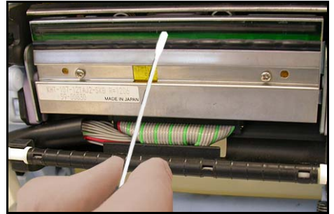
Figure 6-1, Cleaning the print head
