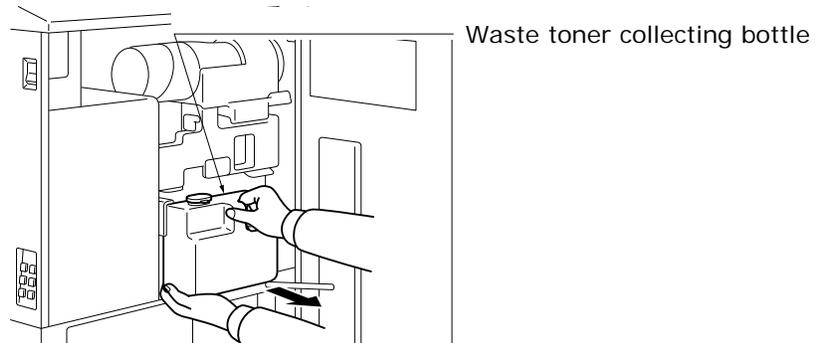
3. Remove the sealing cap from its storage position on the waste toner collecting bottle.
