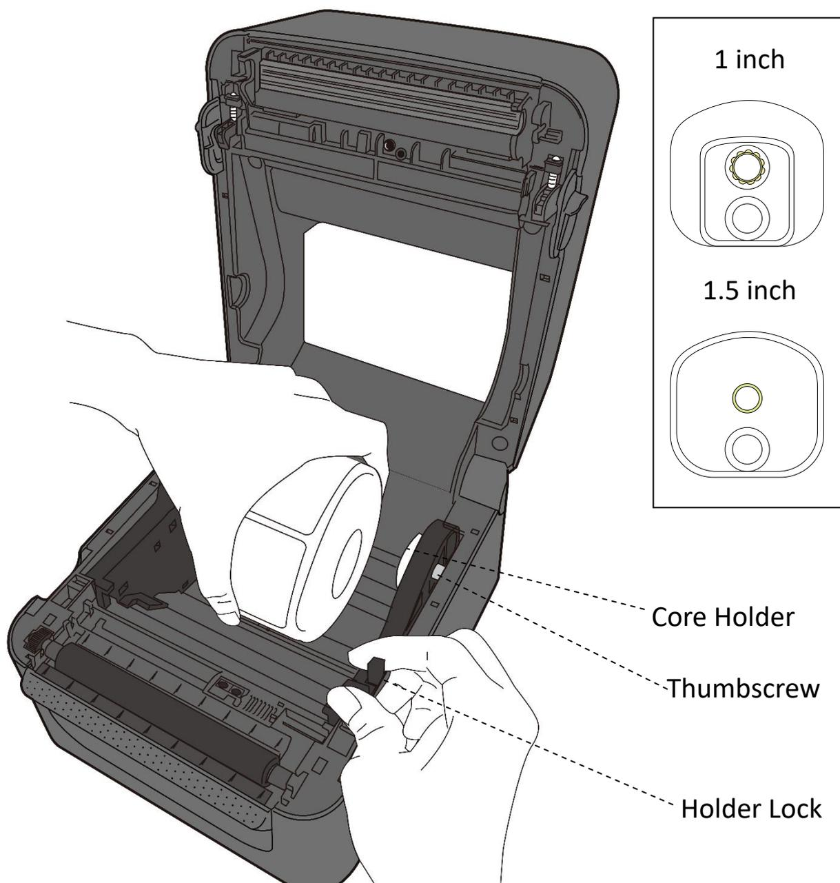
3. Pull the media until it reaches out of the printer. Thread the media under the media guides.
