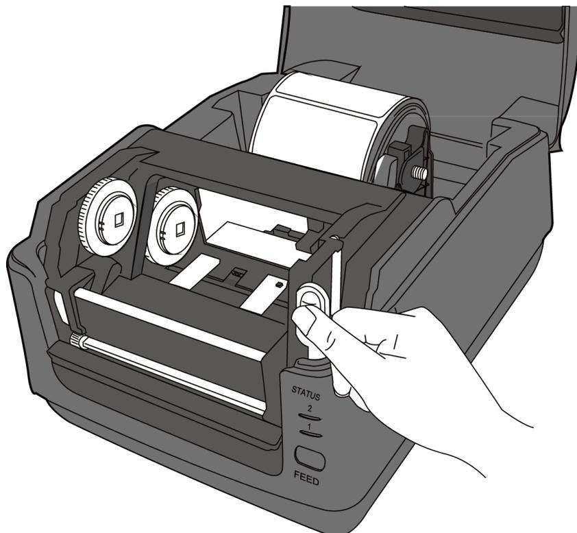
3. Lift the printer module to reveal the **Supply Wheel**.
