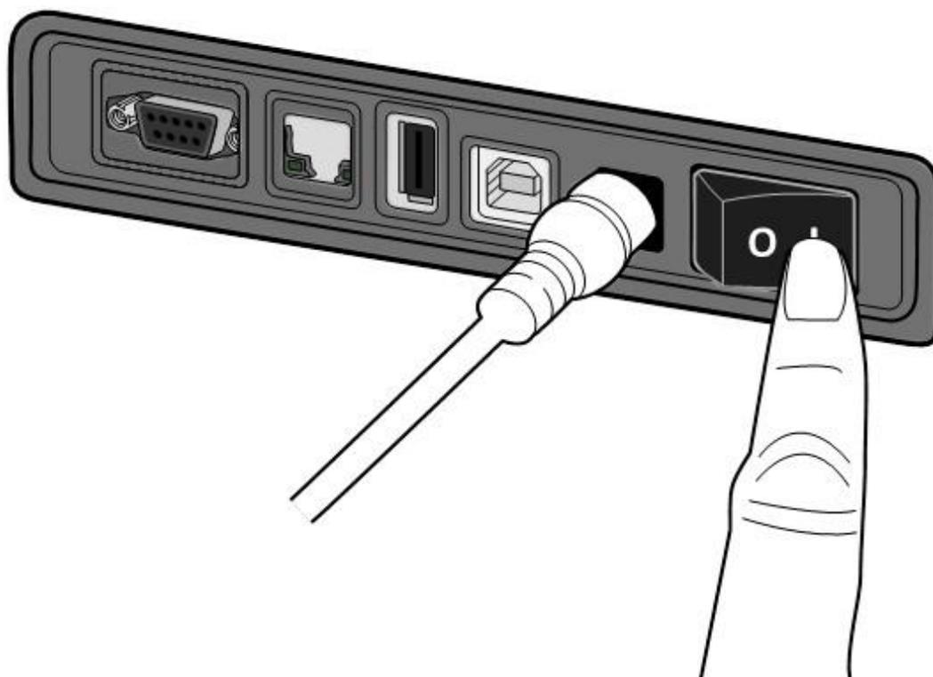
2. Both status lights illuminate solid orange for a few seconds, and then LED 2 goes out, while LED 1 turns to solid green.
