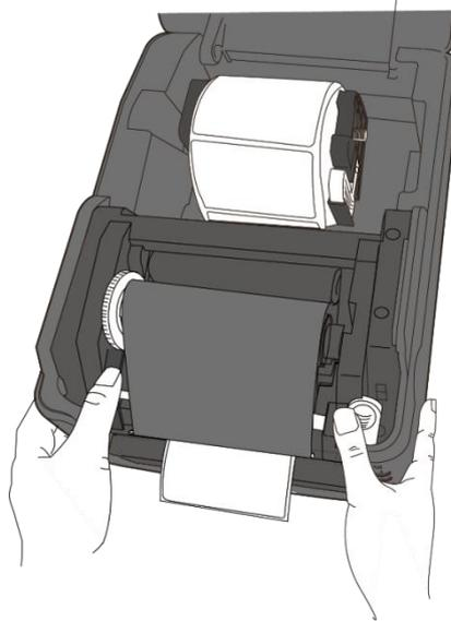
7. Rotate the **Take-Up Wheel** to straighten the ribbon and reduce its wrinkles.
