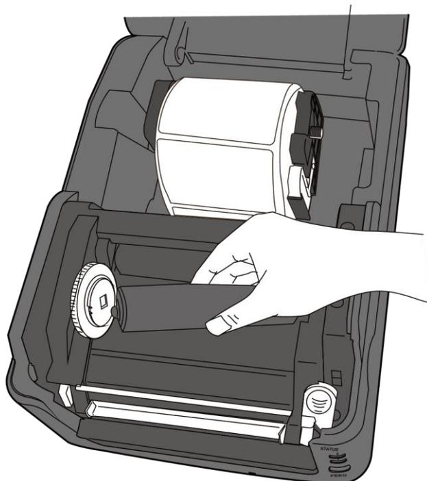
5. Pull the ribbon from the supply roll and tape it on the empty ribbon core.
