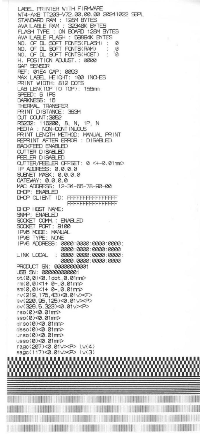
**1. LABEL PRINTER WITH FIRMWARE (MODELLO STAMPANTE E VERSIONE FIRMWARE.)**
