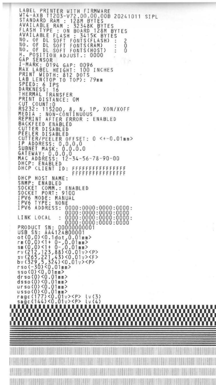
**1. LABEL PRINTER WITH FIRMWARE (IMPRESORA DE ETIQUETAS CON FIRMWARE)**
