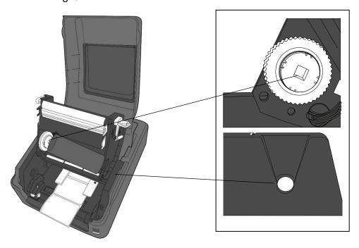
To load the take-up roll, set the empty ribbon core on the core adapter shaft. Then, align the notches on the left side of the roll to the hole on the take-up wheel and place the other end of the roll into the hole on the right.
