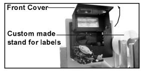
2. Release the purple Head Lock lever by pushing it downwards. The print head assembly will be lifted up to allow label loading.
