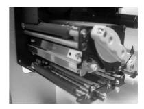
3. Pull the Print Head Release Latch. The print head will drop downwards.
