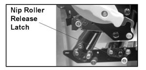
2. Now unlatch the Nip Roller assembly by pressing the release latch as indicated on the right.
