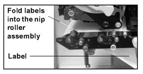
4. Press the Nip Roller assembly upwards and latch it into place.
