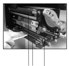
Clean the black rubber rollers: From left: Ribbon Roller, Platen Roller, Feed Roller
