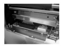
5. Insert the two connectors to the replacement print head. Pull the Head Lock lever and push the print head back into place.
