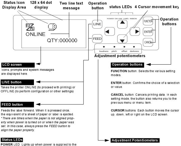
**POWER** LED: Lights up when power is supplied to the printer.
