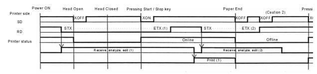
Note: Paper End will be cleared when the Head has been closed. Note 2: An "XOFF" transmission will be executed when receiving data during the occurrence of an error
