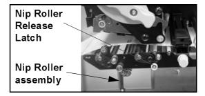
3. Loop the label through the Nip Roller assembly so that two or three labels are hanging freely under the label guide.
