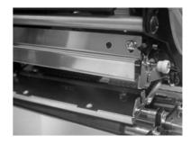
4. Pull the print head outwards and disconnect the two connectors attached to it.
