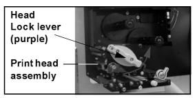
3. Insert the carbon ribbon in the ribbon feeder shaft. Push the ribbon roll inwards all the way, with the ribbon winding in a counterclockwise direction, as shown. Pull the ribbon around the print head assembly so it reaches the Ribbon Take-up Shaft. Note: For maximum print quality and printer durability use genuine SATO carbon ribbons.
