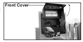
2. Pull the purple Head Lock lever upwards in a counterclockwise direction. The print head assembly will be lifted up to allow ribbon loading.
